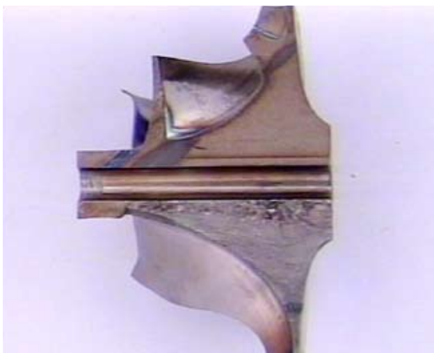
Image 3 / Broken centrifugal compressor after use in a turbocharger
