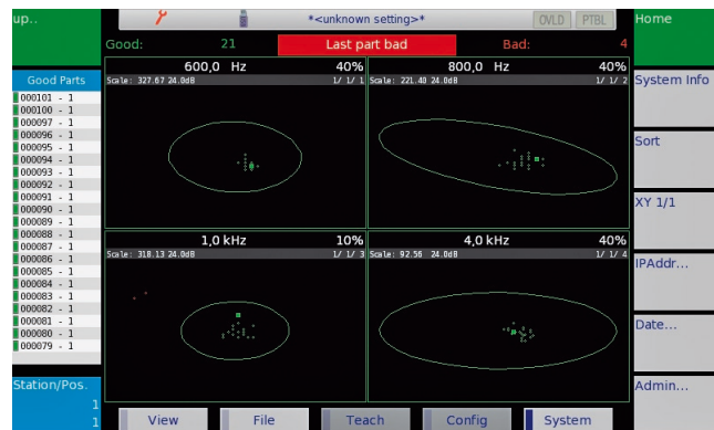
Sorting mode "BubbleGate" in the new Q500-module
