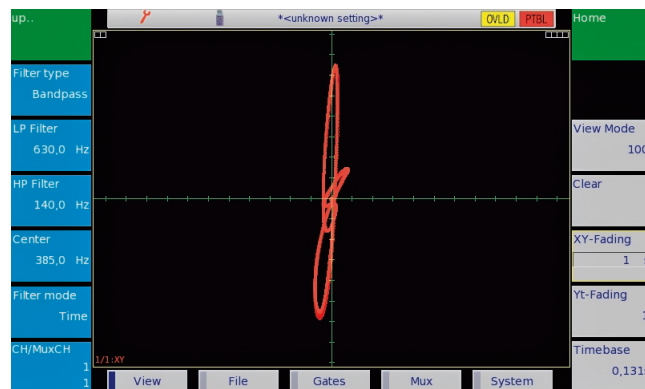
XY display during crack detection
